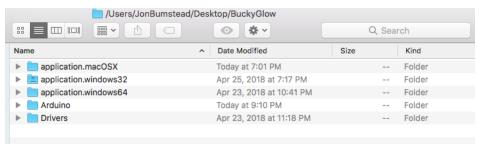
The Bucky Glow has an Arduino Nano with CH340 USB bus convert chip, so the first thing you need to do is download the driver. Double click on the "Drivers" folder, and then choose either "Mac" or "Windows" to install the driver. Follow the instructions for the driver download. If you have problems, use the following links instead:
